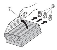
7 Firmly grip the color drum cartridge (®) and remove the protective tray (®) by sliding it toward you.
